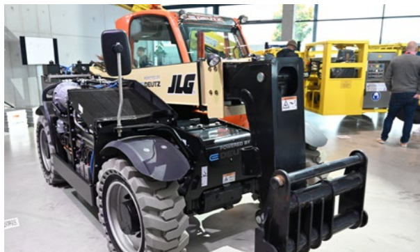
A quiet worker: the JLG telehandler powered by an electric drive from DEUTZ.
